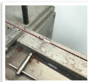
Fine peeling test
